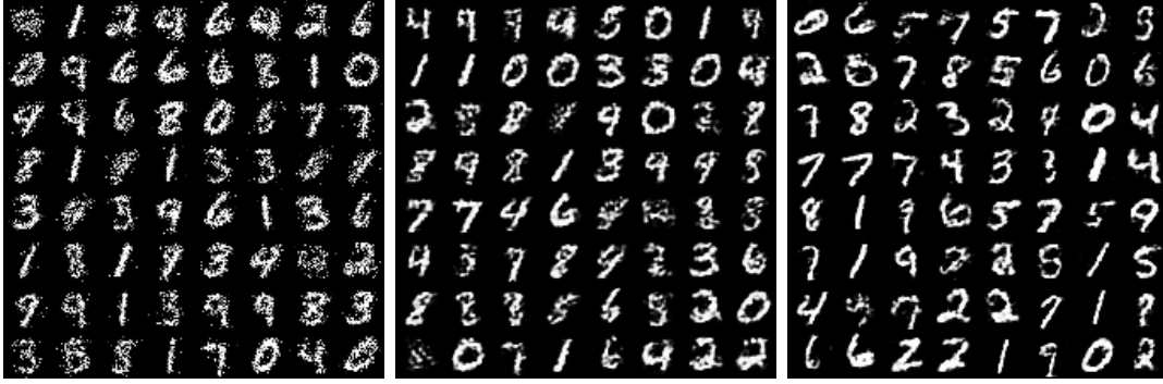
Figure 5.2: The samples at the left are drawn from P_X . Those in the middle are drawn from P_2 , and those at the right are drawn from P_3 . “Cleaning” the samples from P_X using an autoencoder improves the samples, but decoding samples drawn from an SPN modeling the hidden representation of the autoencoder produces even better results.
